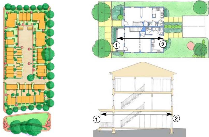
D-58 Left: By raising the elevation of the middle of the block, each building has a zero-step entry from the parking area. Top right: Site detail shows the zero-step entry from the parking area. Bottom right: Cross-section illustrates grading with a raised porch on the street and a zero-step entry from the parking area.
