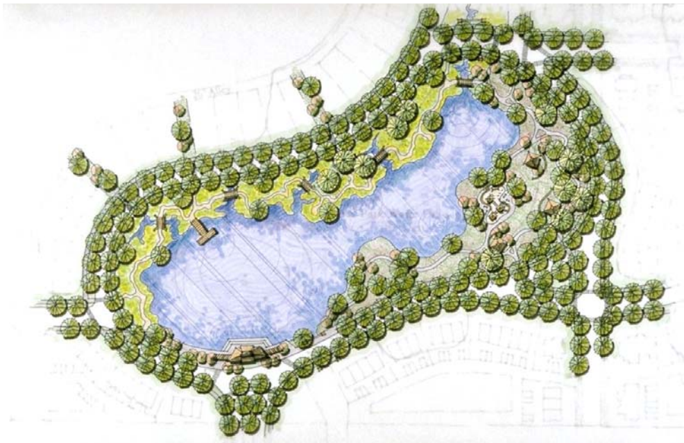
D-47 This water feature was designed as part of a stormwater management system. It also provides attractive views for the blocks which front it and amenities for the neighborhood.
