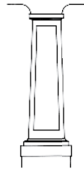
Tapered, Paneled Box on Pier
