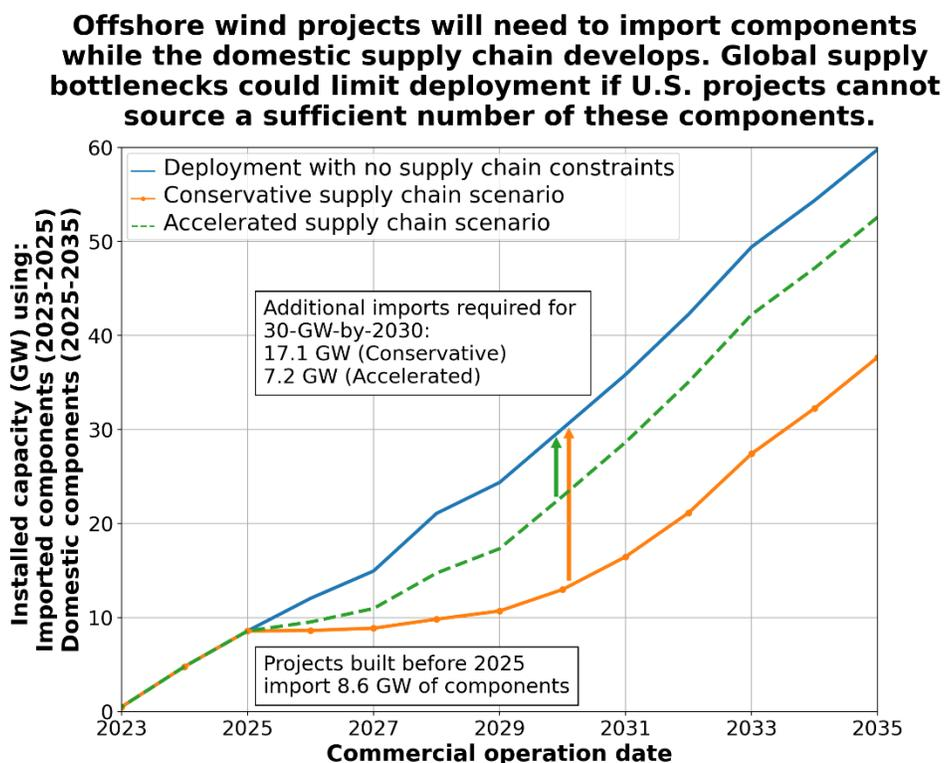
**Figure 18. The time required to plan, permit, and construct offshore wind factories results in limited manufacturing capacity in the mid-2020s, which would need to be met by imported components to meet the 30-GW-by-2030 deployment target.**
