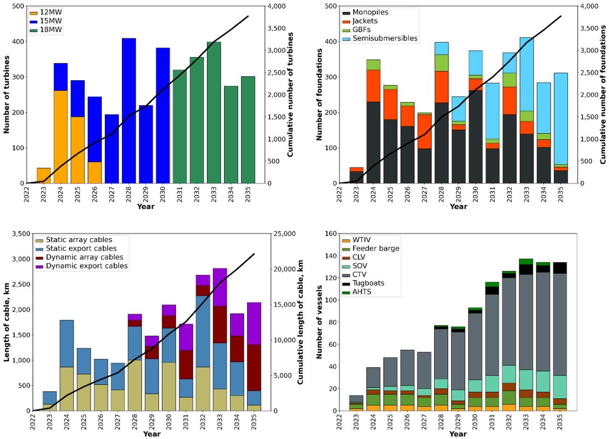
**Figure 2. Annual and cumulative component demand for (clockwise from top left) wind turbines, foundations, vessels, and cables. Figure from Shields et al. (2022)**
