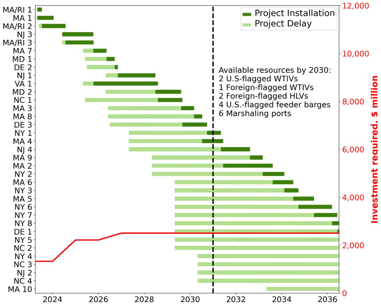
**Figure 9. Deployed fixed-bottom capacity and project delays for the Baseline scenario. Total investment in marshaling ports, WTIVs, and HLVs are also shown.**
