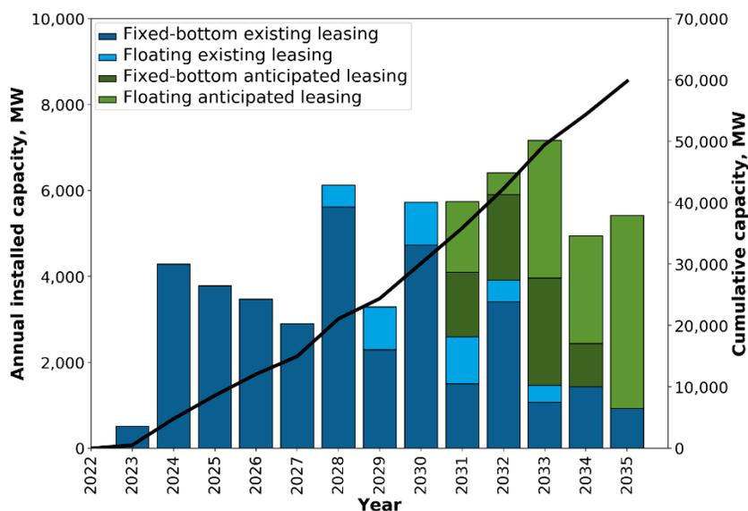
**Figure 1. Annual and cumulative installed capacity for existing and anticipated lease areas.** *Figure from Shields et al. (2022)*
