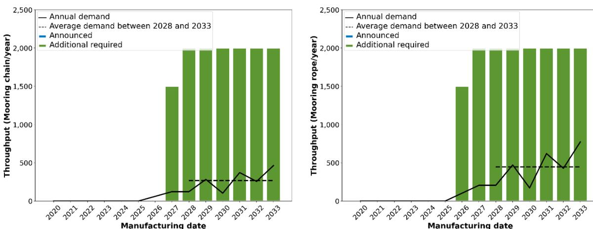
**Figure A8. Comparison of average annual demand and potential production throughput for the mooring chain (left) and mooring rope (right). The production throughput corresponds to one mooring chain facility and one mooring rope facility that come online by 2030.**
