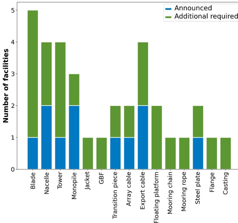
**Figure 13. Total number of major component manufacturing facilities required for a domestic offshore wind energy supply chain. Some facilities have already been announced by manufacturers and additional facilities would be required to meet the anticipated pipeline demand.**
