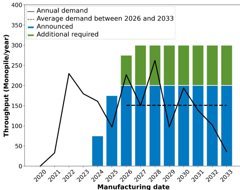
**Figure A4. Comparison of average annual demand and potential production throughput for monopiles. The production throughput corresponds to two monopile facilities that come online by 2030.**
