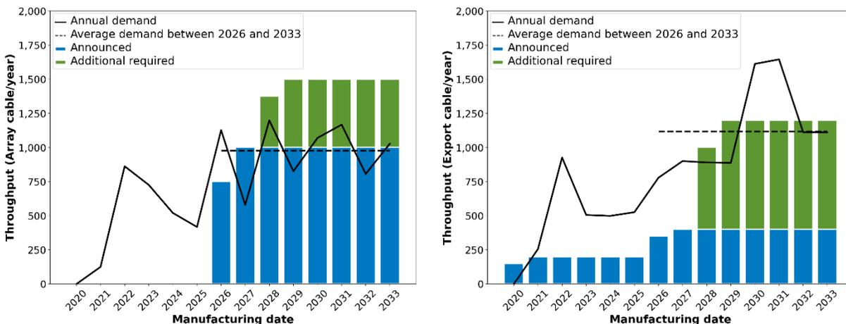
**Figure A7. Comparison of average annual demand and potential production throughput for array cables (left) and export cables (right). The production throughput corresponds to two array cable facilities and four export cable facilities (three HVAC, one HVDC) that come online by 2030.**
