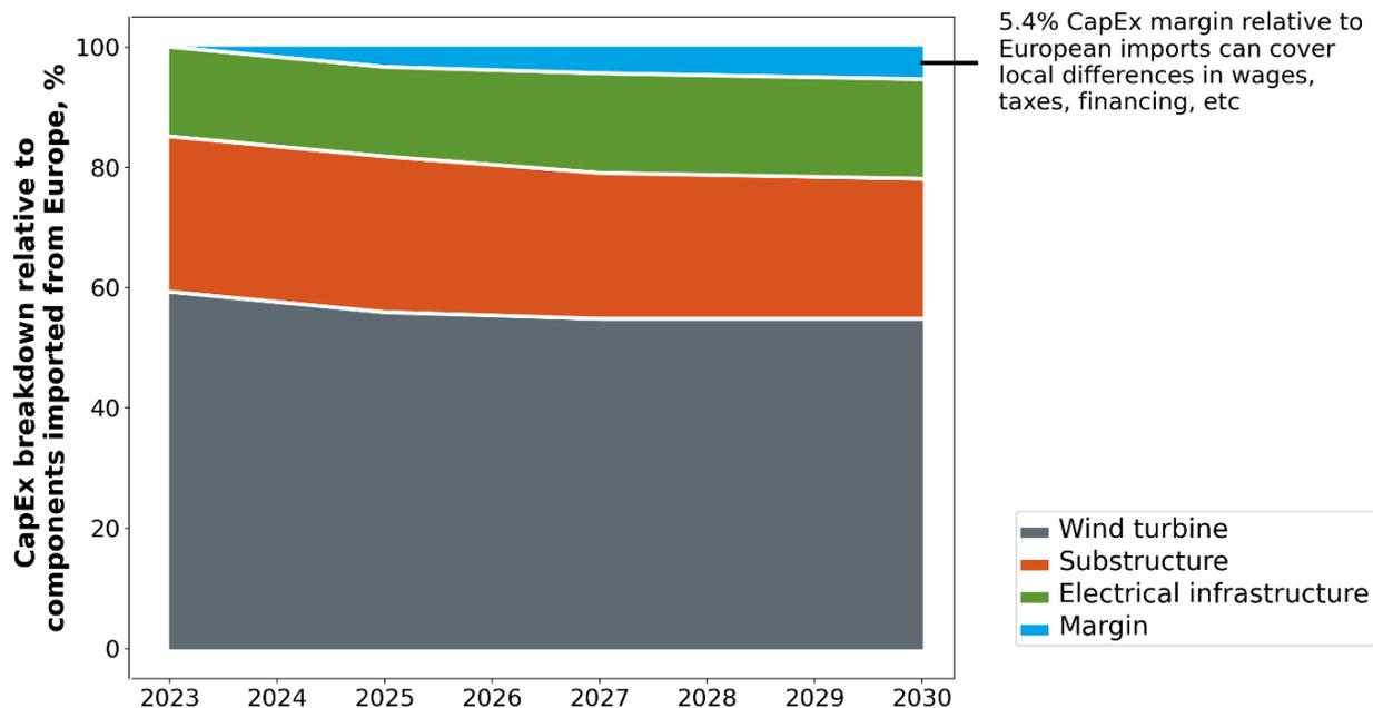
**Figure 23. Percent change in component CapEx for wind turbines (including the blades, nacelle, and tower), substructure (including the monopile and the transition piece), and the electrical infrastructure (cables and substations) for scenarios with expanding domestic manufacturing capacity between 2023 and 2030**
