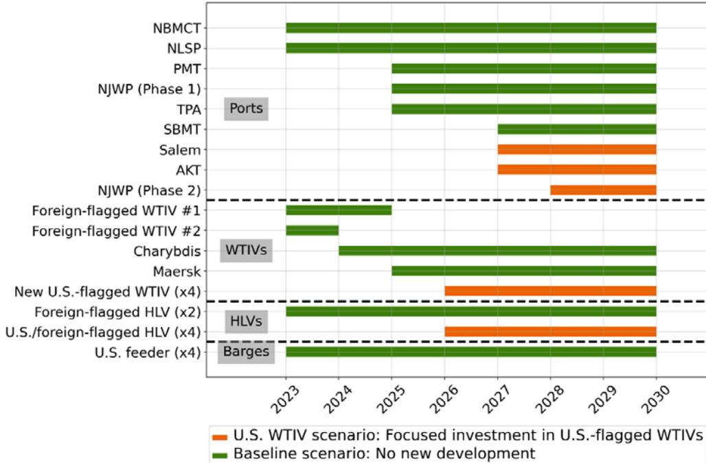
**Figure 7. Availability of marshaling ports, WTIVs, HLVs, and feeder barges in the U.S. WTIV scenario (with the Baseline scenario shown as a reference).**
