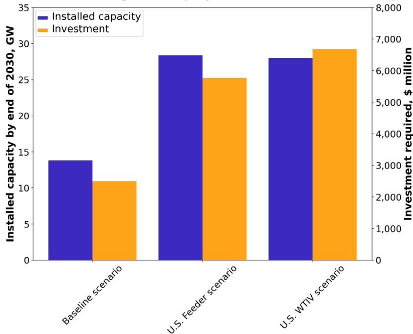
**Figure ES4. Installed fixed-bottom offshore wind capacity by 2030 and investment required for different port and vessel scenarios.**
