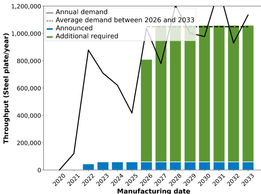
**Figure A9. Comparison of average annual demand and potential production throughput for steel plates. The production throughput corresponds to two steel plate facilities that come online by 2030.**
