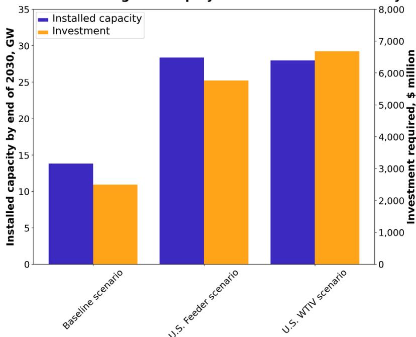
**Figure 12. Summary of installed capacity and capital investment required for the Baseline, U.S. WTIV, and U.S. Feeder port and vessel scenarios**
