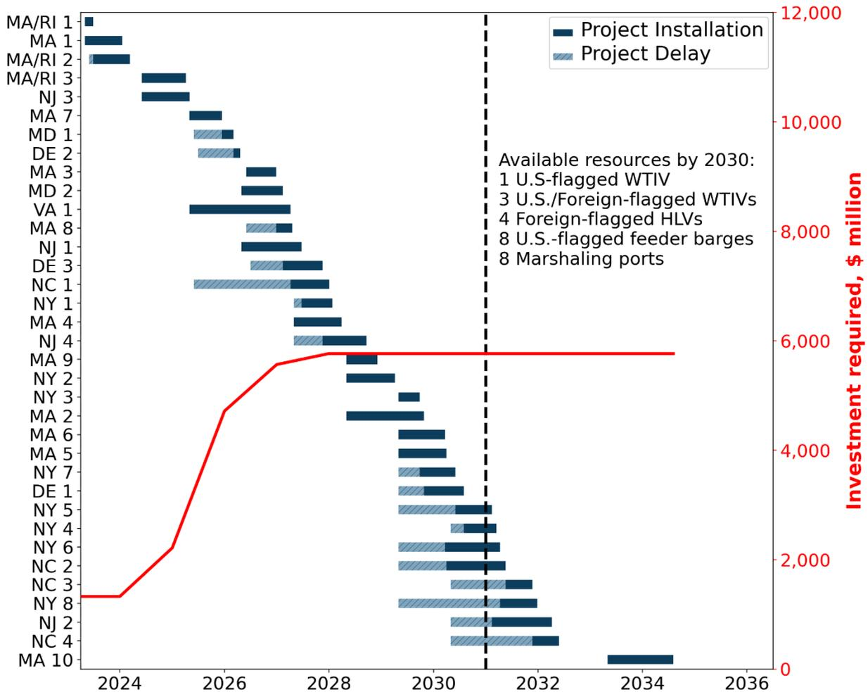
**Figure 11. Deployed fixed-bottom capacity and project delays for the U.S. Feeder scenario. Total investment in marshaling ports, WTIVs, and HLVs are also shown.**
