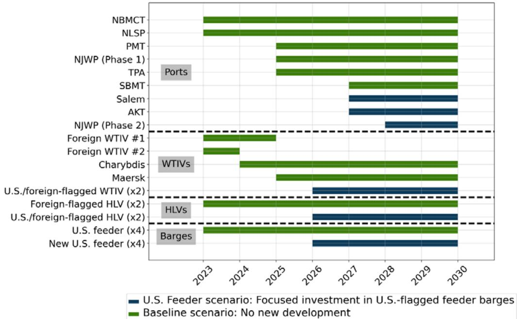
**Figure 8. Availability of marshaling ports, WTIVs, HLVs, and feeder barges in the U.S. Feeder scenario (with the Baseline scenario shown as a reference).**
